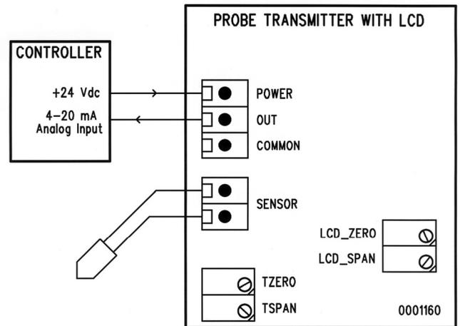
Voltage Connection With Controller 24 Vdc Power
