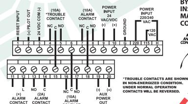
Output terminals are provided for remote accessories such as horns, strobes, remote status indicators and test/reset key switches or push buttons.
