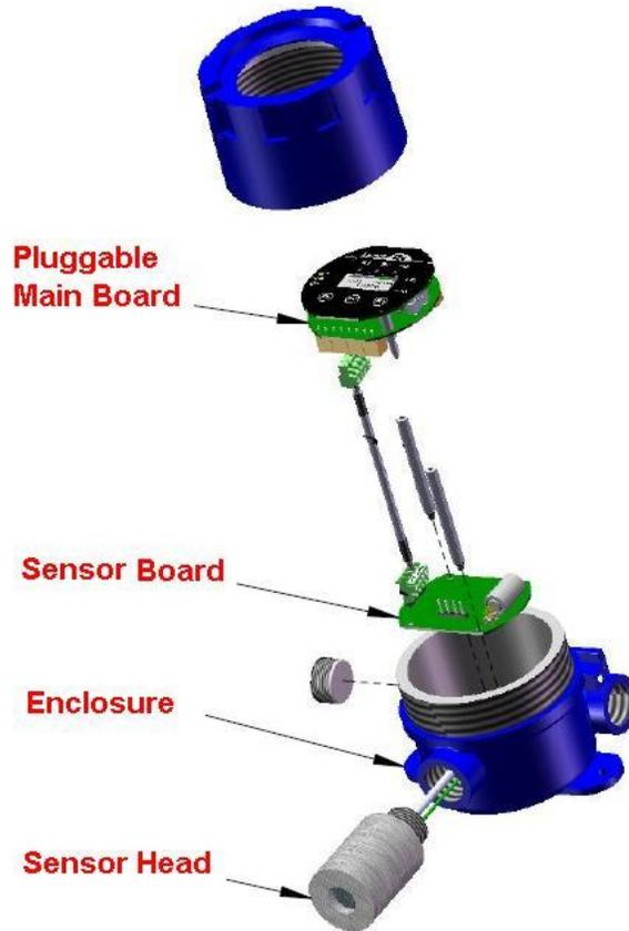
Important: Calibrate the transmitter whenever a component is replaced. But if you replace a smart sensor assembly with a sensor onboard from GES, you don't need to recalibrate the transmitter, as all the calibration information has been stored in the smart sensor board in factory process.
