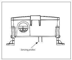
**3** The sensing probes distance to floor is 1 mm (0.04") on lowest leg setting and 26.5 mm (1.04") on highest leg setting.
