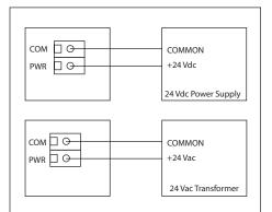
To prevent electrical shock or equipment damage make all connections before applying power. Connect 24 Vac/Vdc to PWR & COM terminals.
