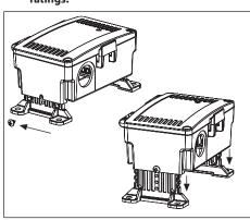
The legs have five pre-set heights. To adjust, remove screws from both legs. Pull/push the legs to the desired height, and re-insert screws.
