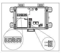
**5** Make all connections in accordance with national and local codes. Use 14-22 AWG shielded wire and do not locate the device wires in the same conduit with wiring used to supply inductive loads such as motors. The device is reverse voltage protected and will not operate if connected backwards.
