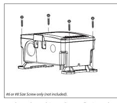
Secure by applying a silicone adhesive to the mounting feet and placing the sensor in the area to be protected. For more permanent installations, fasten the sensor using the holes provided in the mounting feet.
