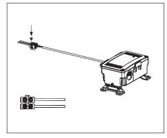
Route the cable to desired location. Mount the terminal block using a screw or adhesive. Make sure sensing probes do not contact any surface.
