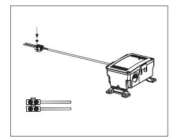
If channel 2 is remote spot detection, route the cable to desired location. Mount the terminal block using a screw or adhesive. Make sure sensing probes do not contact any surface.
