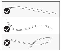
The cable may be laid in a straight line or in a serpentine configuration. Be careful not to kink cable.
