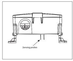
The sensing probes distance to floor is 1 mm (0.04") on lowest leg setting and 26.5 mm (1.04") on highest leg setting.
