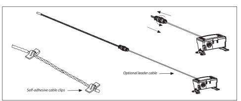
If Channel 2 is Conductivity Cable, Once laid in place, secure using the self-adhesive cable clips provided. For best results adhere clips at each end of the cable first. Clips are provided to secure cable approximately every 1.5 m (5').
