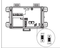
All jumpers are factory set. Improper positioning will cause device to be in constant alarm state. Spot = SPOT position Remote Spot = SPOT position Conductivity Cable = COND position
