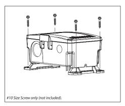
Select a suitable installation area to mount the device. Secure to the floor using silicone adhesive or with a #10 screw (not provided) using the integrated mounting holes.
