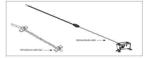
Uncoil the conductivity cables and once laid in place, secure using the self-adhesive cable clips provided. For best results adhere clips at each end of the cable first. Clips are provided to secure cable approximately every 1.5 m (5'). Repeat operation for the second conductivity cable on channel two.
