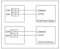
**8** To prevent electrical shock or equipment damage make all connections before applying power. Connect 24 Vac/Vdc to PWR & COM terminals.
