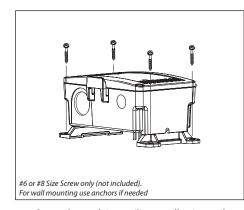
Secure by applying a silicone adhesive to the mounting feet and placing the sensor in the area to be protected. For more permanent installations, fasten the sensor using the holes provided in the mounting feet.
