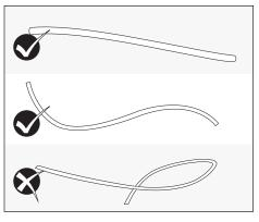
The cable may be laid in a straight line or in a serpentine configuration. Be careful not to kink cable.
