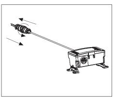
3 If the device was ordered with a leader cable, the conductivity cable can be disconnected to assist in installation. To remove, twist connector counter-clockwise and pull apart.
