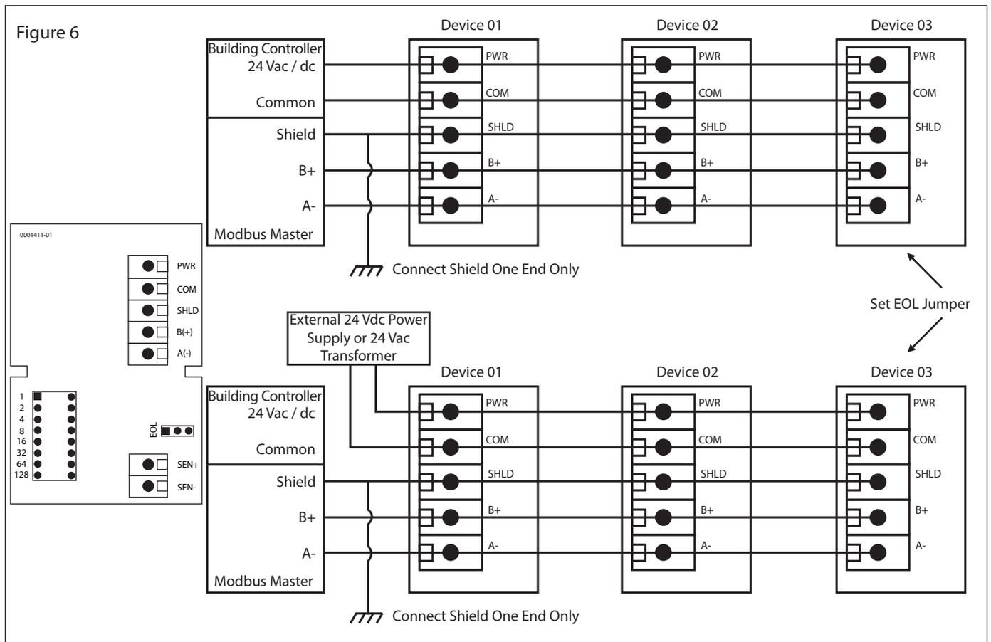
B+ terminals. This device includes a network termination jumper and will connect the resistor correctly on the PCB. Simply move the PCB jumper to the EOL position as shown in Figure 7 and no external resistor is required. The ground wire of the shielded pair should be connected to earth ground at the end of the network and the master is not grounded. Do not run bus wiring in the same conduit as line voltage wiring.
