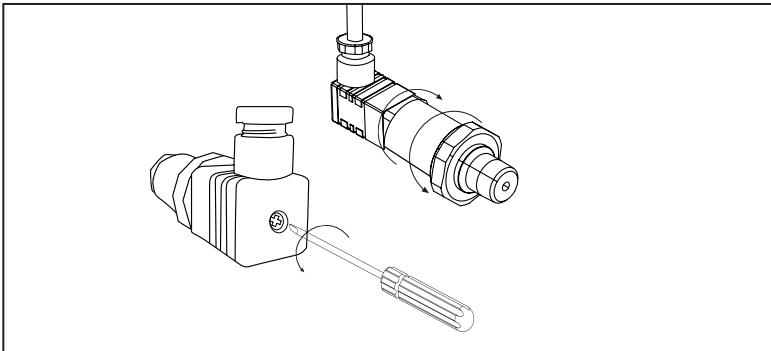
2. Install the sensors into the system plumbing (use 3/4" hex to tighten"). Tape the electrical termination to avoid water infiltration
