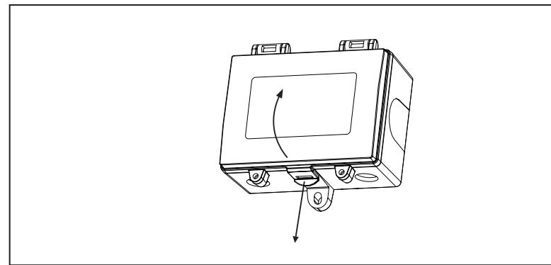
A 1/2" NPT threaded connection hole is provided in the left side of the enclosure as shown in Figure 3. Screw the EMT connector or cable gland connector in until tight. See Figure 4. It is recommended that weatherproof conduit or cable gland fittings be used. The F style enclosure includes 1/2" NPT to M16 thread adapter and cable gland fitting.
