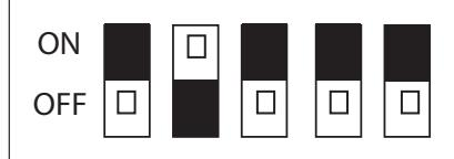
DIP switch setting for Bi-directional (-10 to +10psi) operation..
