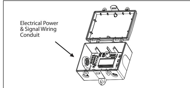
Two security screws are provided which can be installed to help secure the cover once settings and wiring connections are complete.
