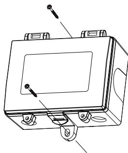
Ensure there is enough space around the unit to make the electrical connections and that it is within an acceptable distance for the length of remote sensor cables. Avoid locations with severe vibrations or excessive moisture. The enclosure has
