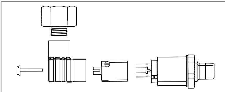
4. Feed wires through a flexible or EMT conduit and insert them into the DIN C connector.
