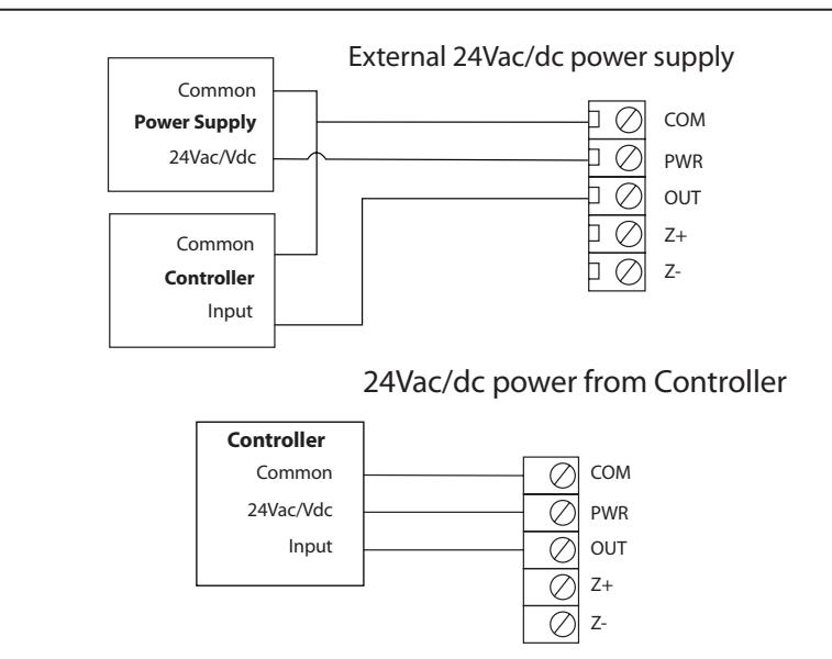
Voltage (0-10V or 0-5V) wiring setup when using a Remote Zero Switch Command. **Switch Common only and do not apply voltage to Z+ terminal.**
