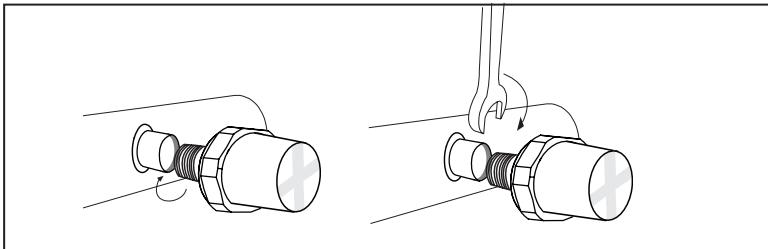
3. Separate the terminal block parts for wiring as shown below
