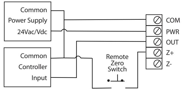
Current 4-20mA is on a 3-wire or loop powered circuit. When using a Remote Zero Switch command **requires Z+ voltage passing thru switch and return signal back to Z- terminal.**
