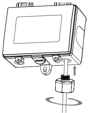
9. Wire the sensor on the terminal block located inside the transmitter. The terminal is removable to ease the wiring step
