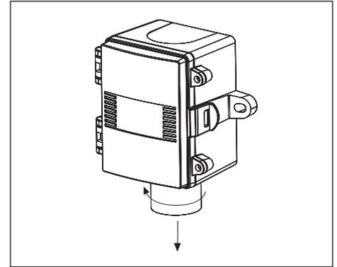
**3** Unscrew the sensor hub from bottom of the enclosure..
