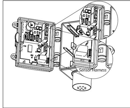
**2** Disconnect power wires. Unplug sensor harness from main PCB.
