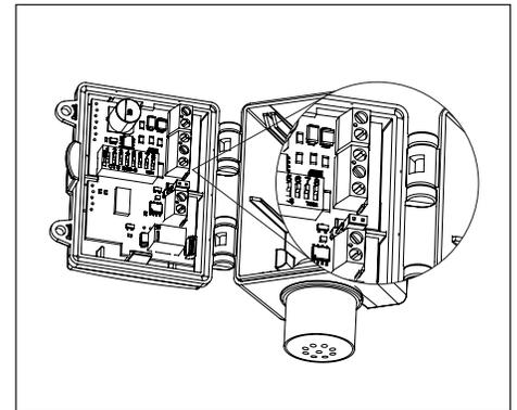
**6** Reinstall power wires and apply power.
