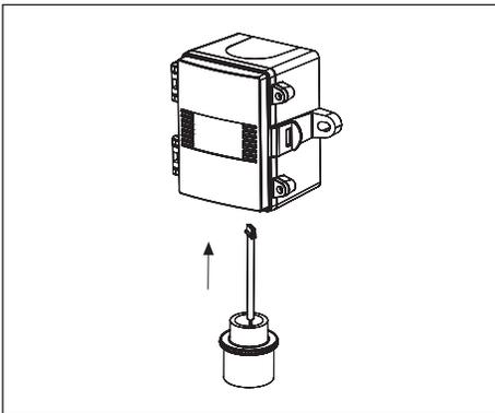
**4** Install replacement module by inserting harness and screwing sensor hub into the bottom of the enclosure.
