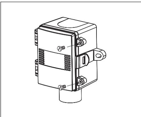
**7** Close enclosure and reinstall security screws (if applicable).
