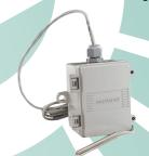
The single point strap-on temperature transmitter incorporates a precision platinum RTD encapsulated in a 6 mm (0.236") OD, 304 stainless steel probe and is available in various lengths. All probes provide excellent heat transfer, fast response and resist moisture penetration. A transmitter that provides a high accuracy signal with excellent long term stability, low hysteresis and fast response is available with various ranges.
