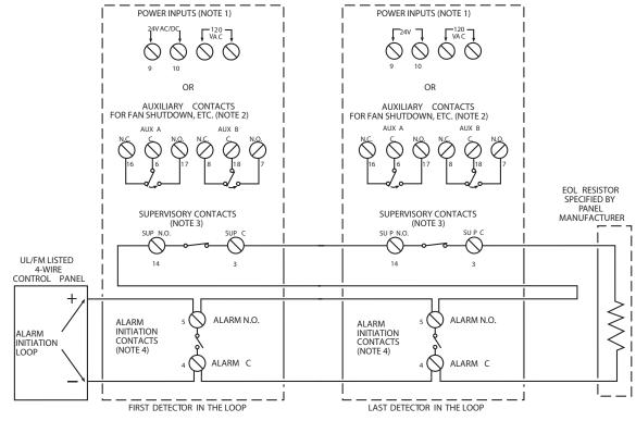
**NOTE 1:** 24V Power Inputs accept a non-polarized 24VDC or 24VAC 50-60Hz. 120VAC Power Inputs accept only 120VAC 50-60Hz. Connect power source to appropriate terminals of each detector. See specifications for additional power supply information.
