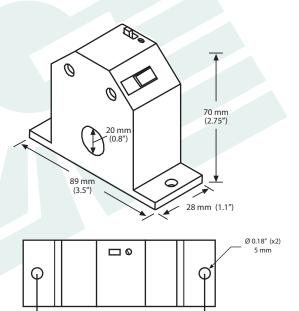
67.2 mm (3″) Solid Core CS-425 Series Current Switch
