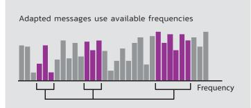
MESH network operates along with other wireless technologies in the building by dynamically using the best available communication frequencies. This patented technology minimizes the likelihood of being interfered by or interfering with other wireless systems.
