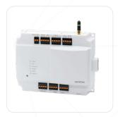
GWBU is a base unit for wireless network transmitters. On this network, all transmitters are communicating with GWBU over the air, with measurement data converted to Modbus TCP/IP, Modbus RTU or 0...10 V analog outputs (6x) for the requirements of BMS or other systems. Wired measurements can be read over Modbus to BMS via inputs (6 px).
