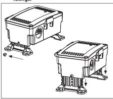
The legs have five pre-set heights set by the holes in the leg. To adjust leg height, remove the screws. Pull/push the legs to the height desired, and re-insert screws and tighten.
