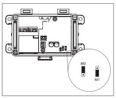
Only for models with 2 relays, set the operation jumper. M0 position = Relay 1 & 2 Activate on water detection and trouble M1
