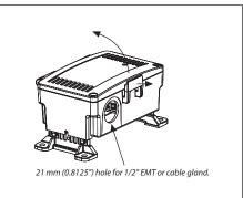
**3** Open the cover by pulling slightly on the latch on the enclosure and at the same time pulling up on the cover.
