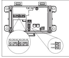
Make all connections in accordance with national and local codes. Use 14-22 AWG shielded wire and do not locate the device wires in the same conduit with wiring used to supply inductive loads such as motors. The device is reverse voltage protected and will not operate if connected backwards.
