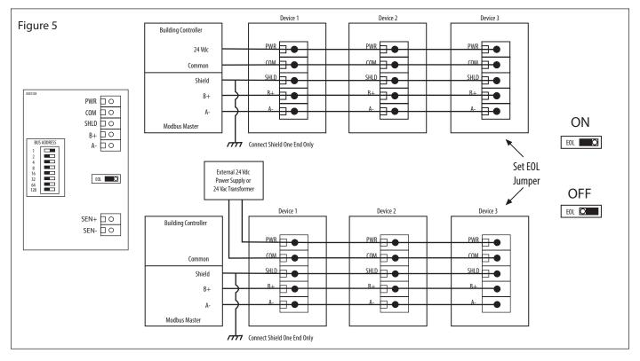
B+ terminals. This device includes a network termination jumper and will connect the resistor correctly on the PCB. Simply move the PCB jumper to the EOL position as shown in Figure 8 and no external resistor is required. The ground wire of the shielded pair should be connected to earth ground at the end of the network and the master is not grounded. Do not run bus wiring in the same conduit as line voltage wiring.
