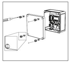
Remove the cover by using a standard or Phillips screwdriver to loosen the four screws. As the screws are captive type, complete removal of the screw from the cover is not required.
