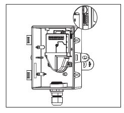
Insert new sensor. Plug harness from sensor into connector on PCB, note the connector is polarized to prevent incorrect installation.
