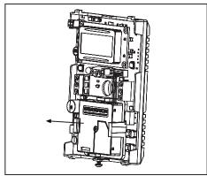
Lift sensor out of clip housing
