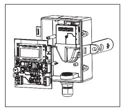
Carefully lift and remove the PCB main board. Set aside.
