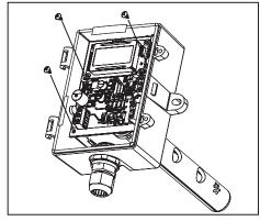
Remove the three PCB screws using a Phillips screwdriver.
