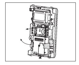
Unplug the sensor harness from the main board. To remove the sensor from the holding clip gently push clip away from one side of the sensor.
