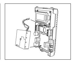
To install new sensor, insert one side of sensor into clip housing under top clip and push sensor down until opposite top clip secures sensor to PCB. Plug harness from sensor into connector on PCB, note the connector is polarized to prevent incorect installation.
