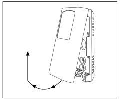
Use the screwdriver to pry each bottom corner if nevessary. Tip the cover away from the base and set aside.
