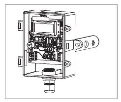
Ensure the power to the unit has been switched off before beginning the replacements of the sensor. A small Phillips screwdriver will be required.
