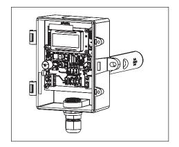
Place PCB board back in place. Tighten 3 security screws.
