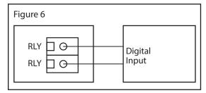
An optional alarm NO relay output is available on the RLY terminals. The relay output is completely isolated. The relay contacts may be connected to a controller Digital Input (DI) for status monitoring or used to directly control an alarm or ventilation fan. Do not exceed the device contact ratings. In some cases, a separate control relay may be used between the relay output and a large fan for example. See Figure 6.
