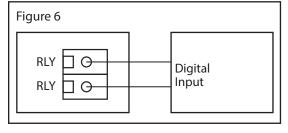
An optional alarm NO relay output is available on the RLY terminals. The relay output is completely isolated. The relay contacts may be connected to a controller Digital Input (DI) for status monitoring or used to directly control an alarm or ventilation fan. Do not exceed the device contact ratings. In some cases, a separate control relay may be used between the relay output and a large fan for example. See Figure 6.
