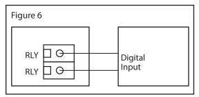
An optional alarm NO relay output is available on the RLY terminals. The relay output is completely isolated. The relay contacts may be connected to a controller Digital Input (DI) for status monitoring or used to directly control an alarm or ventilation fan. Do not exceed the device contact ratings. In some cases, a separate control relay may be used between the relay output and a large fan for example. See Figure 6.
