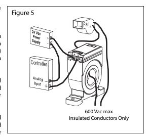
For external CT or multiple wrap applications, ensure the controller is scaled accordingly to obtain correct readings.
