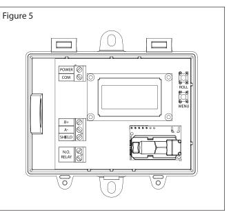
Do not run bus wiring in the same conduit as line voltage wiring or other wiring that switches power to highly inductive loads such as contactors, coils or motors.
