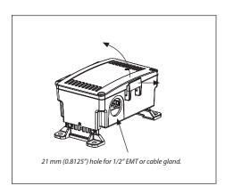
Open the cover by pulling slightly on the latch on the enclosure and at the same time pulling up on the cover.
