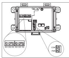
Make all connections in accordance with national and local codes. Use 14-22 AWG shielded wire and do not locate the device wires in the same conduit with wiring used to supply inductive loads such as motors. The device is reverse voltage protected and will not operate if connected backwards.
