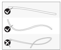
5 The cable may be laid in a straight line or in a serpentine configuration. Be careful not to kink cable.
