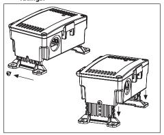
The legs have five pre-set heights set by the holes in the leg. To adjust leg height, remove the screws. Pull/push the legs to the height desired, and re-insert screws and tighten.
