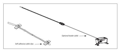
Once laid in place, secure using the self-adhesive cable clips provided. For best results adhere clips at each end of the cable first. Clips are provided to secure cable approximately every 1.5 m (5').
