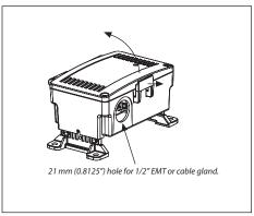
Open the cover by pulling slightly on the latch on the enclosure and at the same time pulling up on the cover.
