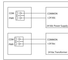
To prevent electrical shock or equipment damage make all connections before applying power. Connect 24 Vac/Vdc to PWR & COM terminals.
