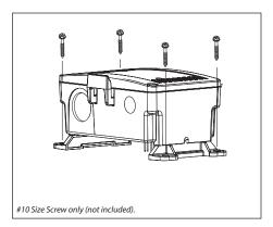
Select a suitable installation area to mount the device. Secure to the floor using silicone adhesive or with a #10 screw (not provided) using the integrated mounting holes.
