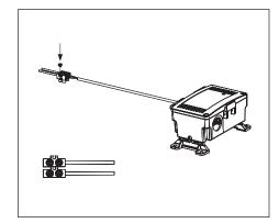
If channel 2 is remote spot detection, route the cable to desired location. Mount the terminal block using a screw or adhesive. Make sure sensing probes do not contact any surface.
