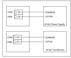
To prevent electrical shock or equipment damage make all connections before applying power. Connect 24 Vac/Vdc to PWR & COM terminals.
