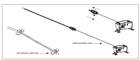
5 If Channel 2 is Conductivity Cable, Once laid in place, secure using the self-adhesive cable clips provided. For best results adhere clips at each end of the cable first. Clips are provided to secure cable approximately every 1.5 m (5').
