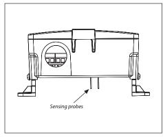
The sensing probes distance to floor is 1 mm (0.04") on lowest leg setting and 26.5 mm (1.04") on highest leg setting.
