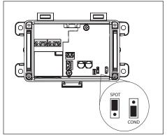
All jumpers are factory set. Improper positioning will cause device to be in constant alarm state.
