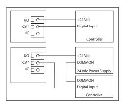
Do not exceed the device contact ratings. The relays are Form C type with both a normally open (NO) and a normally closed (NC) contact. Relay terminals are designated NO, CM\* and NC.
