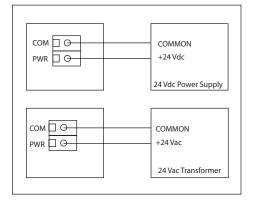
To prevent electrical shock or equipment ndamage make all connections before applying power. Connect 24 Vac/Vdc to PWR & COM terminals.
