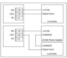
Do not exceed the device contact ratings. The relays are Form C type with both a normally open (NO) and a normally closed (NC) contact. Relay terminals are designated NO, CM\* and NC.
