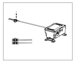
Route the cable to desired location. Mount the terminal block using a screw or adhesive. Make sure sensing probes do not contact any surface. Repeat for Channel 2 if Remote Spot is selected.
