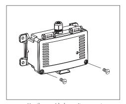
Use the provided security screws to secure the cover.
