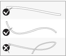
5 The cable may be laid in a straight line or in a serpentine configuration. Be careful not to kink cable.
