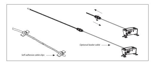
If Channel 2 is Conductivity Cable, Once laid in place, secure using the self-adhesive cable clips provided. For best results adhere clips at each end of the cable first. Clips are provided to secure cable approximately every 1.5 m (5'). NOTE: If the device was ordered with a leader cable, the conductivity cable can be disconnected to assist in installation. To remove, twist connector counter-clockwise and pull apart.
