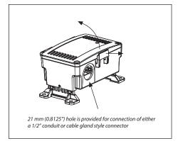
Open the cover by pulling slightly on the latch on the enclosure and at the same time pulling up on the cover.
