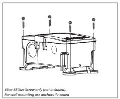
Secure by applying a silicone adhesive to the mounting feet and placing the sensor in the area to be protected. For more permanent installations, fasten the sensor using the holes provided in the mounting feet.
