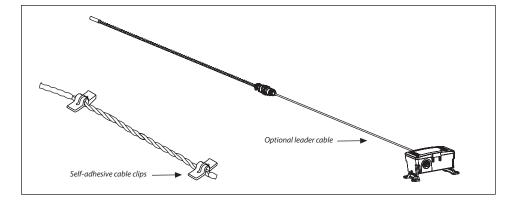
Uncoil the conductivity cables and once laid in place, secure using the self-adhesive cable clips provided. For best results adhere clips at each end of the cable first. Clips are provided to secure cable approximately every 1.5 m (5'). Repeat operation for the second conductivity cable on channel two.
