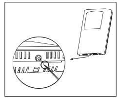
The cover is hooked to the base at the top edge and must be removed from the botton edge first. Use the screwdriver to loosen the security screw. Complete removal of the screw is not required.
