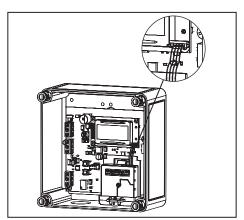
Insert one side of sensor into clip housing under top clip and push sensor down until opposite top clip secures sensor to PCB. Plug harness from sensor into connector on PCB, note the connector is polarized to prevent incorrect installation.
