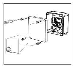
Remove the cover by using a standard or Phillips screwdriver to loosen the four screws. As the screws are captive type, complete removal of the screw from the cover is not required.
