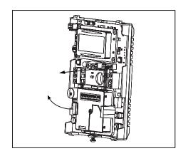
Unplug the sensor harness from the main board. To remove the sensor from the holding clip gently push clip away from one side of the sensor.
