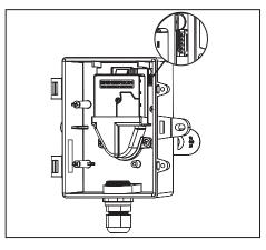
Insert new sensor. Plug harness from sensor into connector on PCB, note the connector is polarized to prevent incorrect installation.
