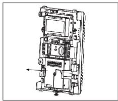
Lift sensor out of clip housing
