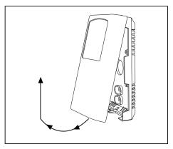
Use the screwdriver to pry each bottom corner if nevessary. Tip the cover away from the base and set aside.
