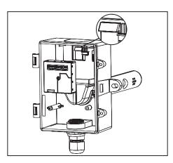
To remove sensor, gently push the tab, while sliding the sensor up and out of the holder.
