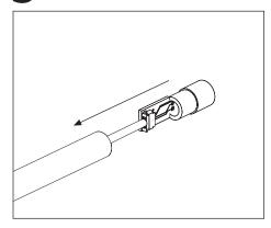
Carefully insert sensor PCB/filter assembly into probe.
