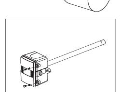
Remove security screws (if applicable) and open enclosure.
