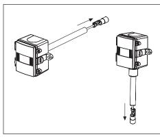
Carefully pull filter from the probe end so sensor PCB is exposed.
