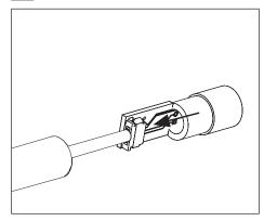
Install replacement module by plugging harness into sensor PCB.
