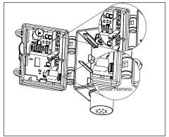
Disconnect power wires. Unplug sensor harness from main PCB.
