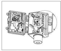
Reinstall power wires and apply power.
