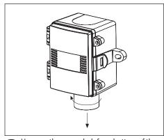
3 Unscrew the sensor hub from bottom of the enclosure..
