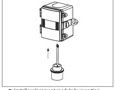
Install replacement module by inserting harness and screwing sensor hub into the bottom of the enclosure.
