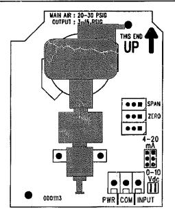
PWR – 24Vac/dc (For ETP-9500, 0-10Vdc only) COM – POWER/SIGNAL COMMON INPUT – 0-10Vdc OR 4-20mA
