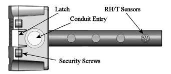
Drill or punch a 1-1/8" or 1-1/4" hole in the duct at the preferred location and insert the probe into the hole to mark the enclosure mounting holes. Remove the unit and drill the four mounting holes. Clean all drilled holes of debris before mounting the device.
